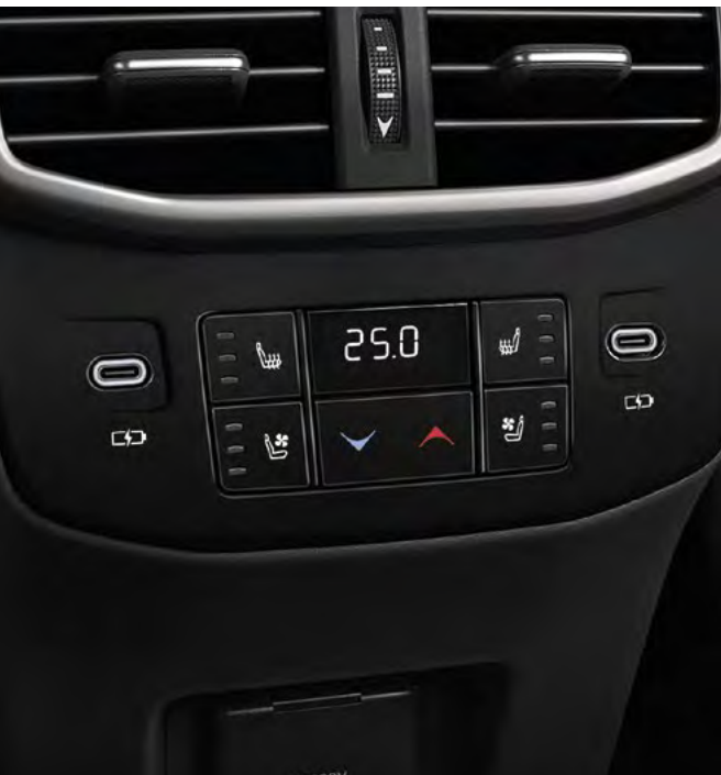
Console rear end: 2 USB Type C charging ports
